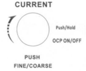
Current Adjustment Knob: Push the voltage adjustment knob and then the voltage meter will flicker, when voltage output can be changed by adjusting the knob. And push the knob again when the meter flikers, then the resolution of the knob rotation can be changed.
